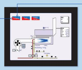
Capable of single servomotor control, modulating gas valve (and optionally VSD) for atmospheric boilers.
