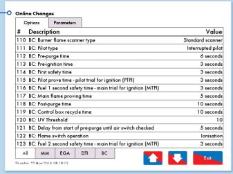
Over 150 options and parameters can be adjusted, providing a sophisticated level of customisation. All of these are viewable while the boiler is online. A selection of these changes can be set while the burner is running, ensuring minimum boiler downtime.
