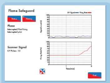
The flame is monitored via UV or IR scanner or ionization probe. The UV scanner can feature self-checking to cover an unmanned boiler house.
