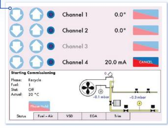
Single Point Change allows a technician to edit the combustion curve without the need of a full re-commission, reducing downtime.
