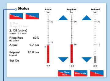
Easily change target set points for both the Required setpoints (used for general ouput) and the Reduced setpoints (used for when less steam or hot water is required).
