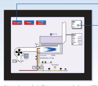
It is much more fuel efficient to run two boilers at 60% than three boilers at 20%. Intelligent Boiler Sequencing (IBS) manages the number of boilers firing at any given time, automatically taking unneeded boilers offline or into standby warming modes to maintain load demand. Users can manage up to 10 boilers.
