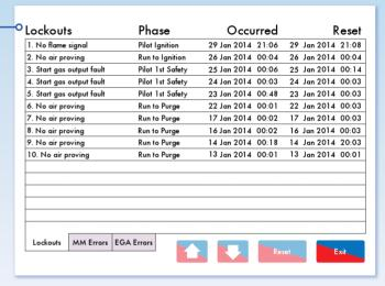
Error and Lockout logs allow engineers to view a history of burner operation to aid in troubleshooting. View the most recent 64 errors and lockouts.
