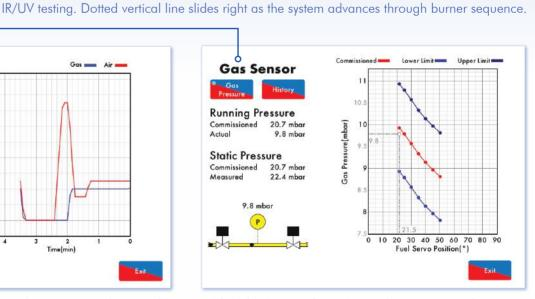
VPS (Valve Proving System) tests the main gas valves to ensure seal integrity and safety.
