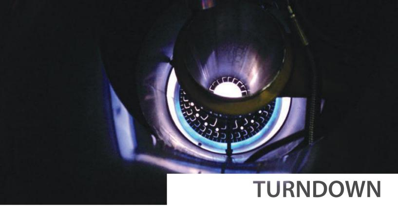
Limpsfield burners provide high turndowns typically between 4:1 and 10:1. This turndown is established by using a split gas head or a spider head design. The split gas head can be used on most applications and provides excellent mixing to maintain good combustion throughout the firing range.
